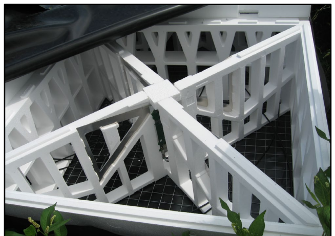
Figure 4-5: LOFAR LBA inverted vee crossed dipole antennas above a ground plane with amplifier on top (left) and a HBA crossed dipole antenna above a ground plane in a dense 4x4 tile array supported by a polystyrene structure covered with weather resistant foil, credit: ASTRON
