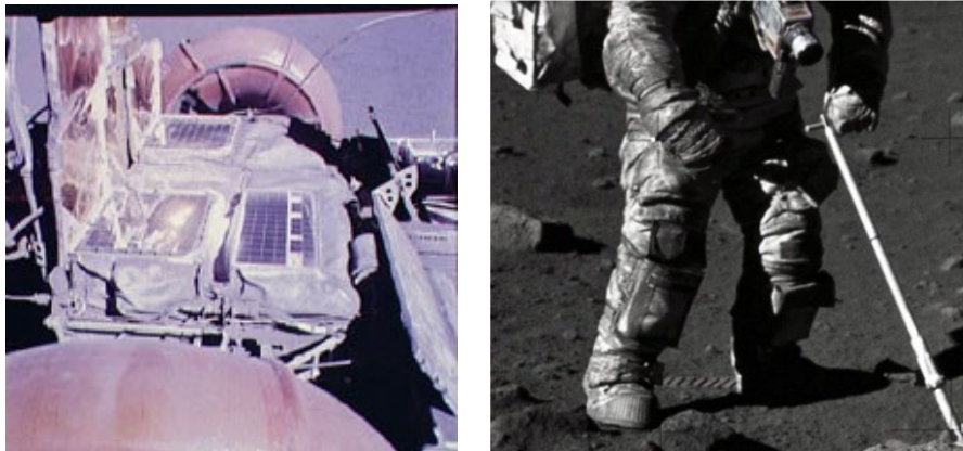
Figure 13-3: Left: Dust on the radiator of the Lunar Roving Vehicle; Right: Impact of lunar dust on the spacesuits of astronauts during Apollo; (credit: NASA)
