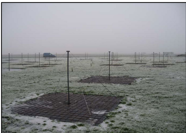
Figure 4-5: LOFAR LBA inverted vee crossed dipole antennas above a ground plane with amplifier on top (left) and a HBA crossed dipole antenna above a ground plane in a dense 4x4 tile array supported by a polystyrene structure covered with weather resistant foil, credit: ASTRON
